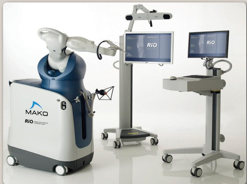
*MAKOplasty Partial Knee Replacement is performed using the robotic arm technology of The Robotic Arm Interactive Orthopedic System (RIO)*
